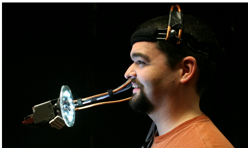
Figure 2: Head-mounted camera and LED light ring
